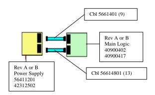
In order to use Revision A or B Power Supply with Revision C PCB, the tech will need to order the connection cables below. (p/n 41998701 9 pin) and (p/n 41998801 13 pin)
