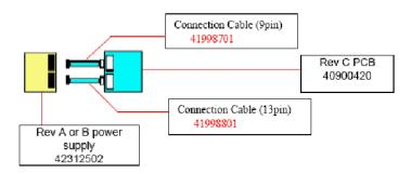
In order to use Revision C power supply with Revision A or B printers, the tech will need to order the connection cables. (p/n 41998701 9 pin) and (p/n 41998801 13 pin)
