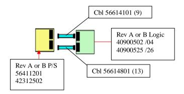
In order to use Revision C power supply with Revision B printers, the tech will need to order the connection cables below. (p/n 41998701 9p) and (p/n 41998801 13p)
