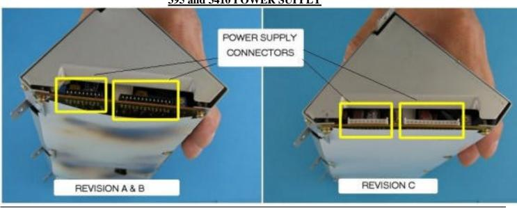
For both rev A and B, the power supply connectors are BLACK. On rev C, they are both WHITE
