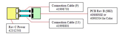
Revision C Power Supply and PCB and cables.
